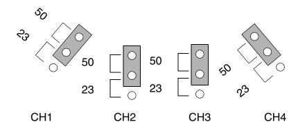
Figure 1-42: Jumpers on the DTGM21
