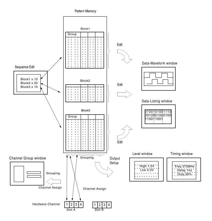
Figure 1-2: Concept of data and window
