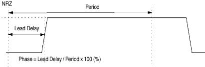
Figure 1-30: Definition of Pulse parameters
