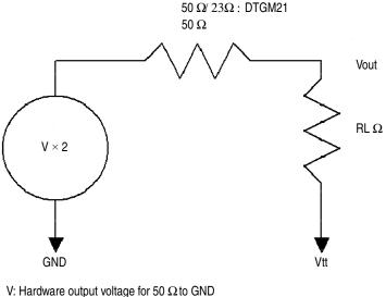
V: Hardware output voltage for 50  $\Omega$  to GND Vout: Output voltage for the termination voltage Vtt and the termination resistor RL  $\Omega$ Source Impedance: 50  $\Omega$  50  $\Omega$  / 23  $\Omega$  (DTGM21only)
