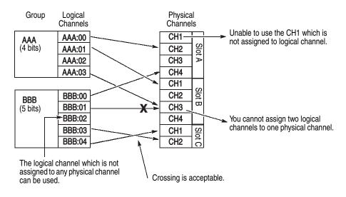
Figure 1-3: Channel assignment
