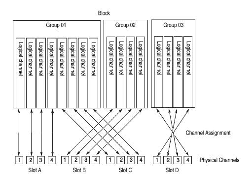
Figure 1-1: Channels, groups, blocks and channel assignment
