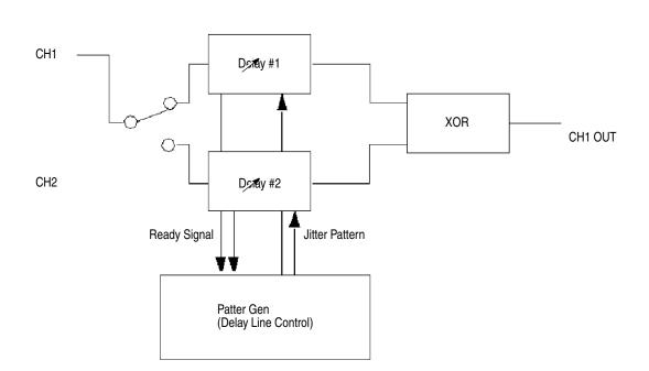
Figure 1-51: Jitter Generation (All pattern jitter)
