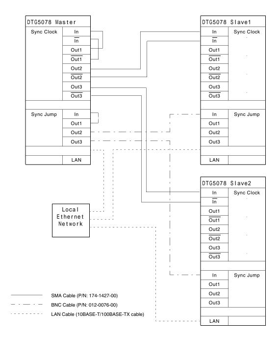
Figure 1-61: Master-Slave cable connection (DTG5078)
