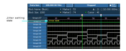
Figure 1-55: Jitter setting state on the Data-Waveform window
