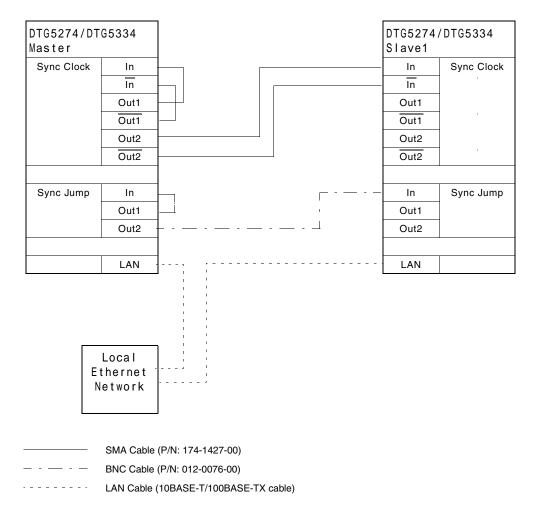
Figure 1-60: Master-Slave cable connection (DTG5274 and DTG5334))
