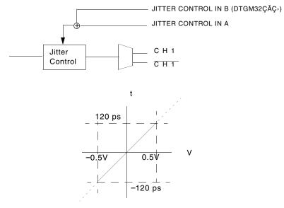
Input Voltage vs. Jitter Amplitude (DTGM 31)
