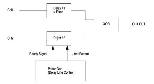
Figure 1-52: Jitter Generation (Partial pattern jitter)
