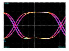
3. Set the oscilloscope controls so that an eye pattern is displayed on the screen.
