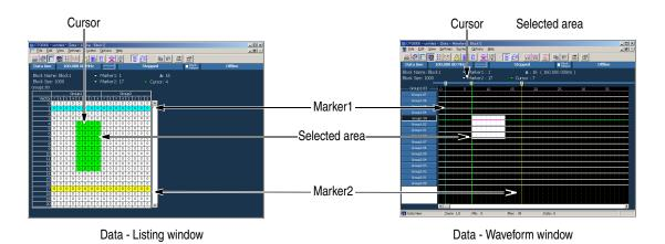
Figure 1-5: Data-Listing window and Data-Waveform window
