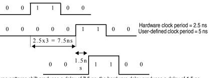
Three patterns shift produces a delay of 7.5 ns; the hardware delay produces a delay of 1.5 ns. This causes a total delay of 9 ns.
